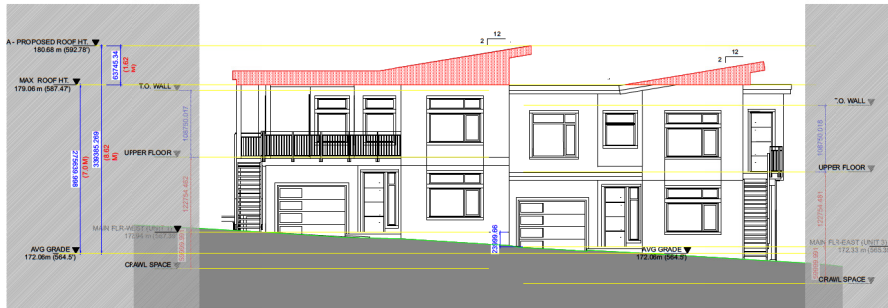
BUILDING A: SOUTH ELEVATION PROPOSED HT.: 8.62 M; MAX. HEIGHT: 7.00 M HEIGHT VARIANCE REQUESTED: 1.62 M ▨ AREA OVER MAX. HEIGHT
