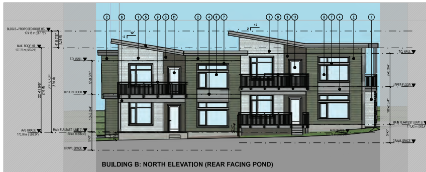
BUILDING B: NORTH ELEVATION (REAR FACING POND)
