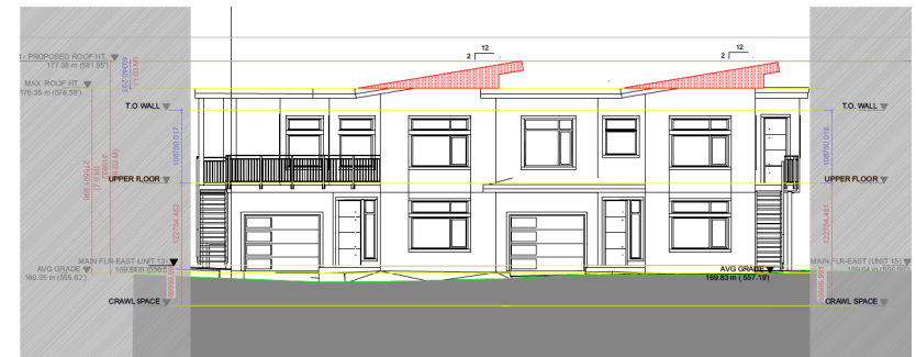
BUILDING D: SOUTH ELEVATION PROPOSED HT.: 8.03 M; MAX. HEIGHT: 7.00 M HEIGHT VARIANCE REQUESTED: 1.03 M ▨ AREA OVER MAX. HEIGHT
