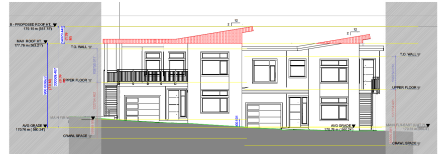
BUILDING B: SOUTH ELEVATION PROPOSED HT.: 8.39 M; MAX. HEIGHT: 7.00 M HEIGHT VARIANCE REQUESTED: 1.39 M ▨ AREA OVER MAX. HEIGHT
